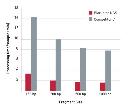
The Bioruptor® NGS efficiently processes up to 12 samples at the same time. Compared to Competitor C, the Bioruptor® NGS requires only 23 minutes to sonicate 12 samples (200 bp), for a time savings of more than 1.5 hrs.
